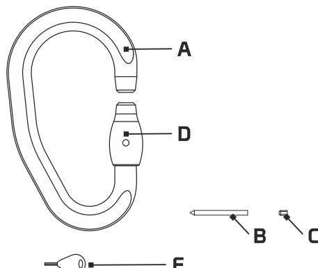
**EN:** (A) Stainless steel body, (B) Stainless steel bar for lanyard locking, (C) Galvanized steel grub screw, (D) Stainless steel gate, (E) Key for removal in case of emergency evacuation (not supplied).
